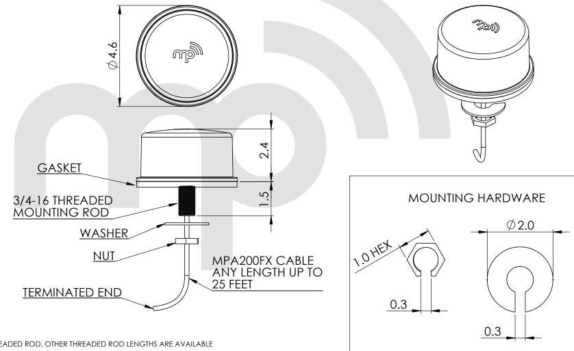
DRAWING SHOWS 1.5" THREADED ROD, OTHER THREADED ROD LENGTHS ARE AVAILABLE
